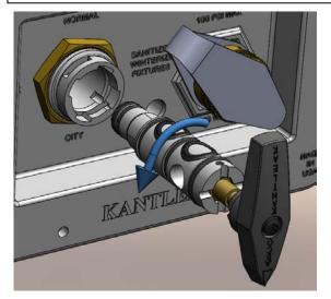
(4) While rotating the handle slowly, pull the valve cartridge out of the valve body. ("click" washer will come out with cartridge if couldn't get out at step 2)
