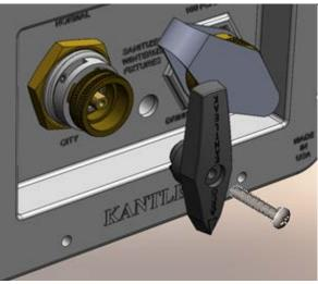
(11) Re-install handle with "new sst" screw in the same position as previously removed. Then rotate the handle 2 full turns in both directions, feeling the click in each
