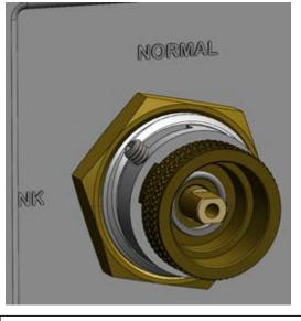
(10) Re tighten the set screw until snug, flush with plastic (this prevents cap from turning)
