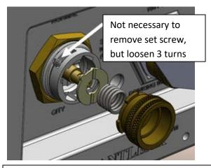
(2) Using supplied 2mm hex key, back off small set screw 3 turns
