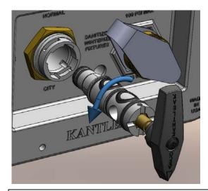
(6) While rotating the handle slowly, push the new valve cartridge into the valve body until fully seated. Stop with the handle pointing to any 1 of the 4 positions
