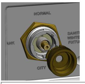
(9) Place spring over valve stem and onto click washer.Align the tabs on the cap, with the slots in the valve body and push onto spring until cap can turn clockwise (approx 1/8 turn) and lock into place.
