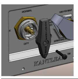
(7) Noting the position the handle is pointing, Remove the handle screw and handle
