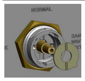
(8) Place "Click" washer, back into valve with the formed, raised side toward the cartridge and the semi-circular locating tab into the internal body groove
