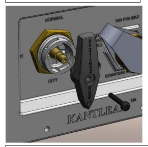
(3) Re-install handle screw and handle back onto the stem of the 4-function, fill valve
